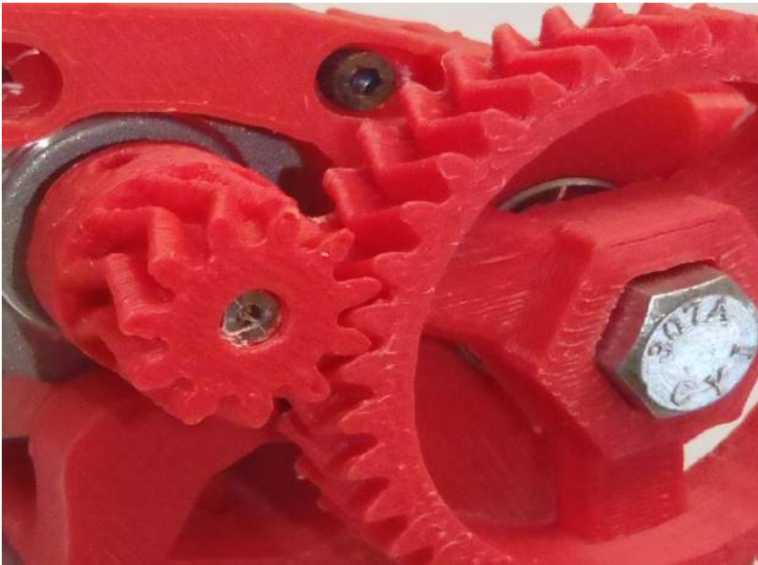
Gear wheels using greater strength of ABS
